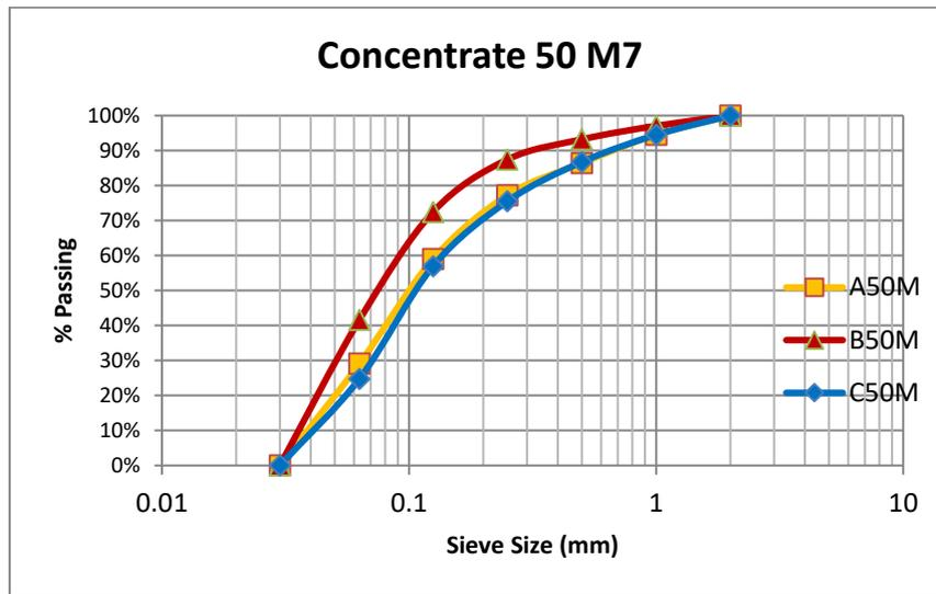
Figure 5: Comparison between the PSD curves of the concentrate samples of the M7.
