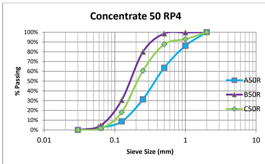
Figure 4: Comparison between the PSD curves of the concentrate samples of the RP4.
