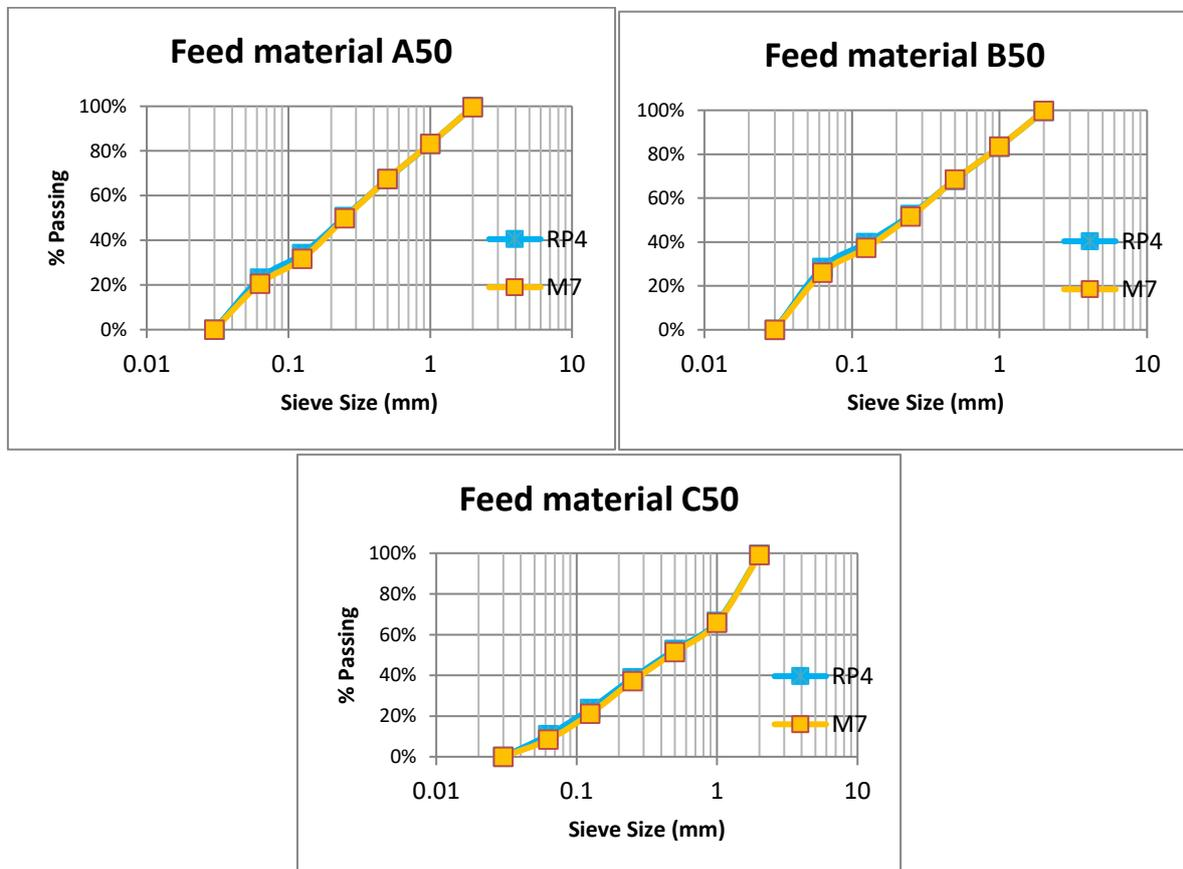
**Figure 1: Comparisons between the PSD curves of the feed of RP4 and M7.**
