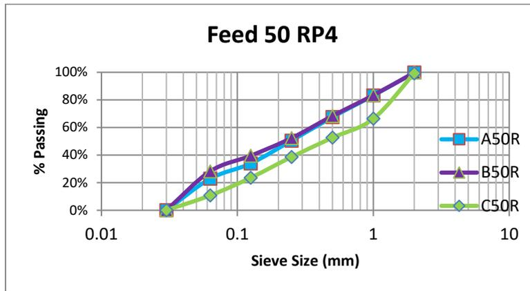
Figure 2: Comparison between the PSD curves of feed sample A50, B50 and C50.
